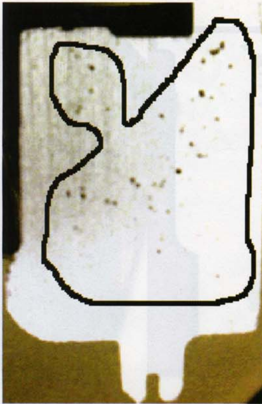
Microporosity in an A380 diesel engine part.
