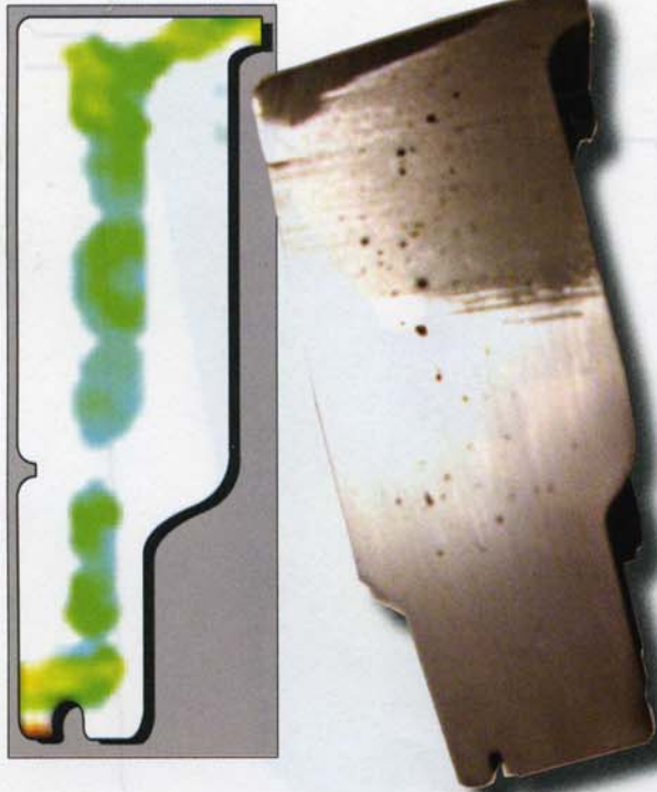
Software can correctly predict the increase in microporosity as shown in this section of an A380 diesel engine part. These images show the part before rotation.
