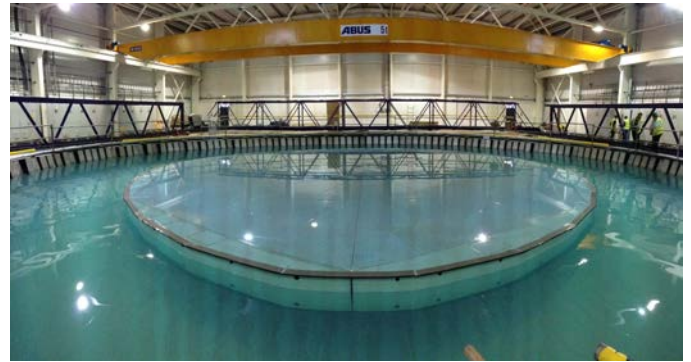
Fig. 11. Basin following completion of the O&M installation and the initial fill with the TLP floor in the raised position.
