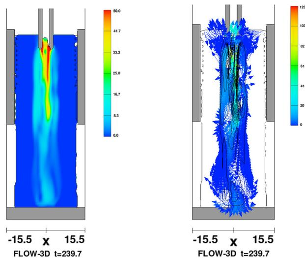
Fig. 4 Calculated velocity contours and vectors inside metallurgical zone  $t=240$  s
