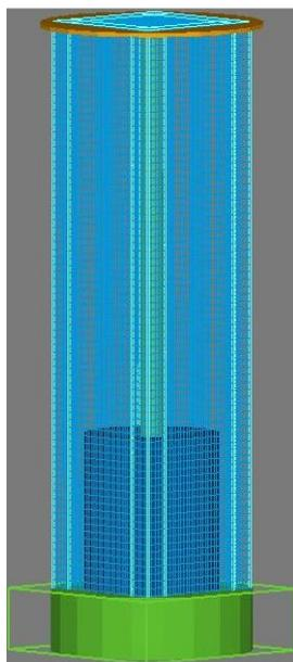
Fig. 2 3D model of fluid region, mold, bottom block and submerged nozzle
