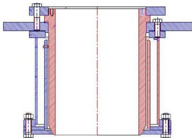
Fig. 1 Cylindrical water cooled mold
