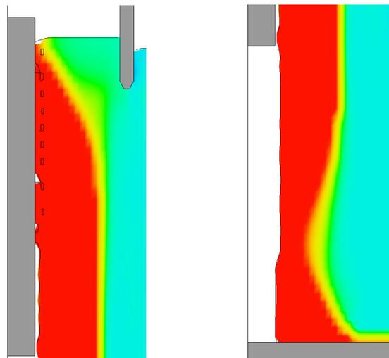
Fig. 6 Details of calculated fraction of solid ratios
