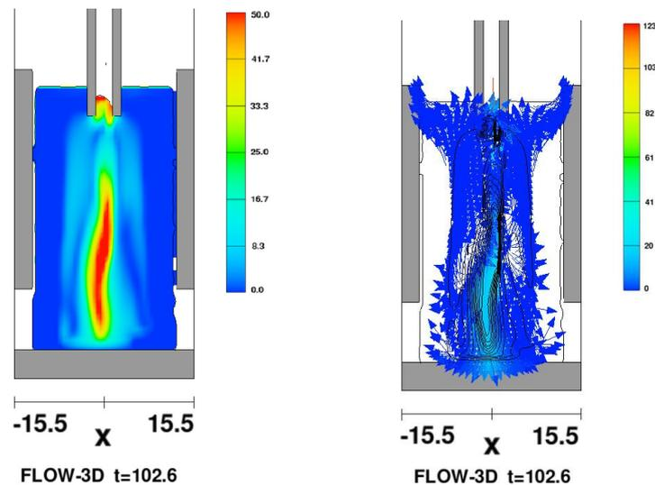
Fig. 3 Calculated velocity contours and vectors inside metallurgical zone  $t=103$  s
