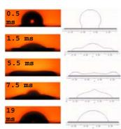
Figures 1a and 1b: Experimental and simulated diameters and profiles of the spreading drop
