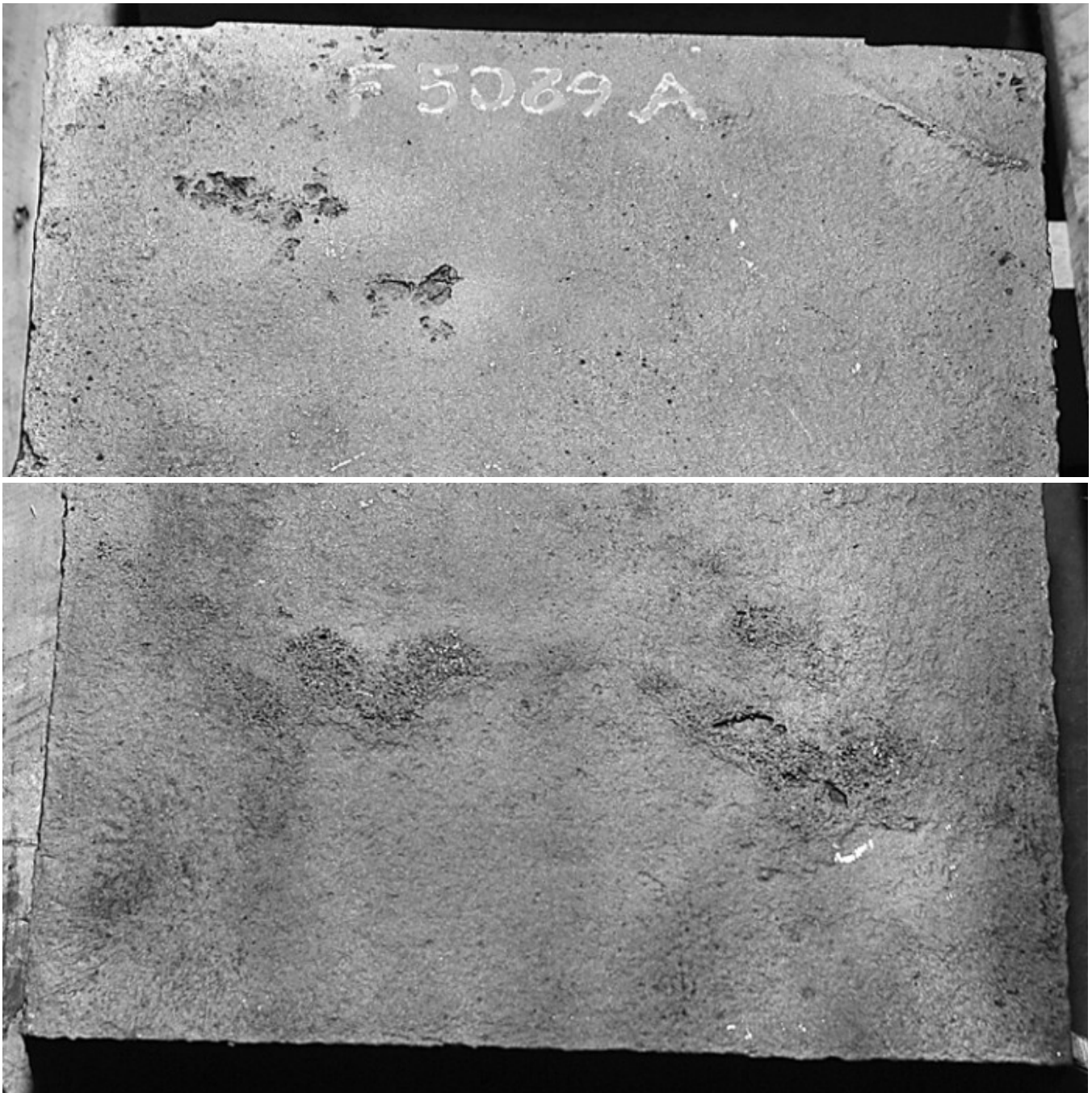
Fig. 3. Close-up views from F5089A showing surface defects resembling a “mold blow”. These defects are commonly termed “Ceroxide”.
