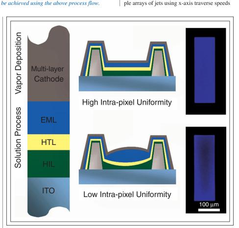
Fig. 2: At left is an architectural cross-section of a solution-processed OLED device. The middle shows a schematic cross-section of high and low intra-pixel uniformity in OLED layers (not to scale) and at right is a corresponding example of blue-subpixel EL images.
