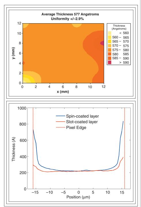
Fig. 3: At top is a thickness contour map of an HIL slot coated on a  $150 \times 150$ -mm bare glass substrate; the coating has a uniformity of ±2.9% of the 577-Å layer. At bottom is shown a stylus profilometer measurement of a subpixel (cross-section), comparing spin vs. slot-coated layer thickness within a subpixel.
