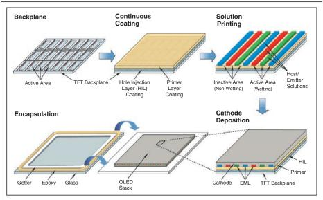
Fig. 1: Solution-coated OLED fabrication can be achieved using the above process flow.
