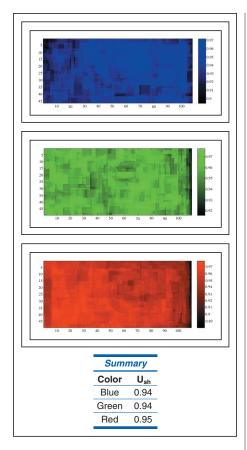
Fig. 6: Shown is a uniformity map of SRU  $(UR_{ii})$  over a large section of a printed AMOLED display and the average SRU  $(U_{sh})$ for each color (table). These SRU values equal or exceed the values reported for commercial AMLCDs. 12
