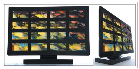
Fig. 7: This prototype AMOLED-TV array was made with DuPont's OLED solution-processing technology and materials and was exhibited at the Society for Information Display's Display Week 2010. The array is composed of 16 4.4-in.-diagonal 55-ppi displays, representing a segment of a 40-in. HDTV.
