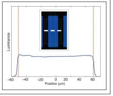
Fig. 5: At left are printed film profiles obtained with a stylus profilometer and a custom automated software analysis program. The inset shows a sample of the raw scan data where a printed row is located next to an unprinted row with identical underlayers. The red dashed lines represent the edge of the pixel. On the right is an example of a luminance intensity plot used to analyze intra-pixel uniformity.
