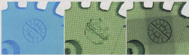
Figure 3 – Finite element meshing of a stereolithography CAD part with fine features. A localized finer resolution captures the details of the part.
