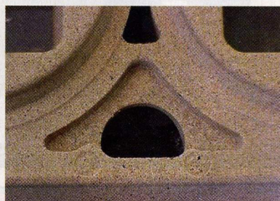
Core prints for castings with internal geometries must be sufficiently vented to avoid core-gas blow defects.
