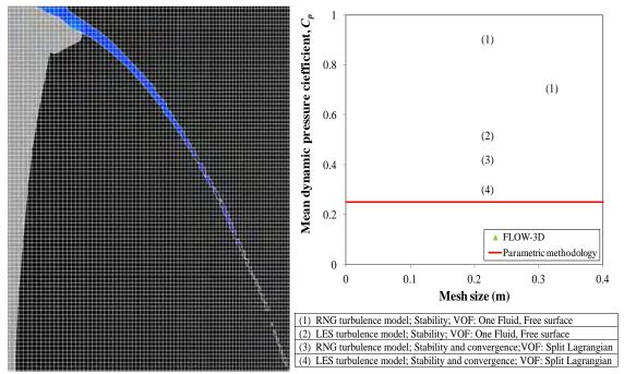
Figure 6. Mesh and sensibility analysis of FLOW-3D.
