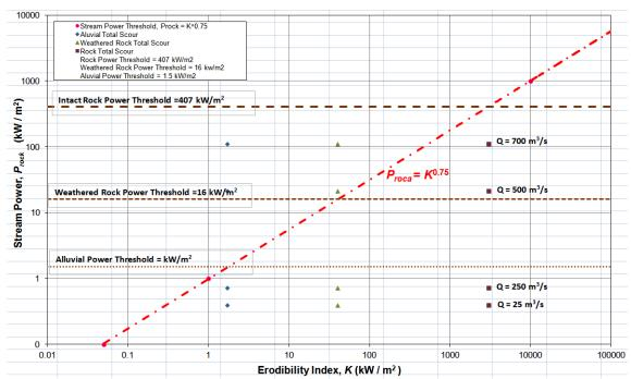
Figure 6. Free surface weir. Stream power of the jet for different flows as a function of the erodibility: alluvial, weathered rock and intact rock indexes (water cushion depth 24 m).
