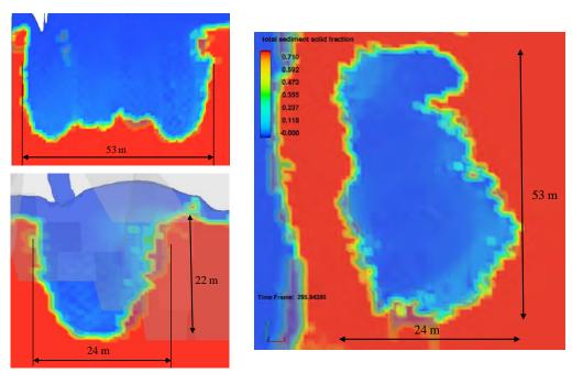
Figure 8. Front, lateral, and top view of the scour due to the free surface weir.
