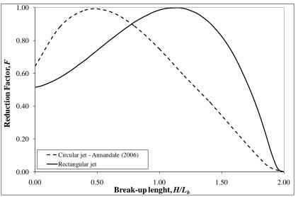
Figure 3. Reduction factor F of fluctuating dynamic pressure coefficient.
