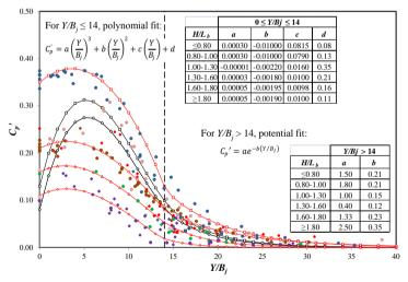
Figure 5. Fluctuant dynamic pressure coefficient,  $C_p$ ', for the rectangular jet.
