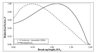
Figure 3. Reduction factor F of fluctuating dynamic pressure coefficient.
