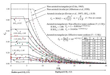
Figure 4. Mean dynamic pressure coefficient,  $C_p$ , for the aerated circular and rectangular jet.
