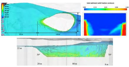
Figure 7. Top, front and lateral views of the scour due to the half-height outlet.
