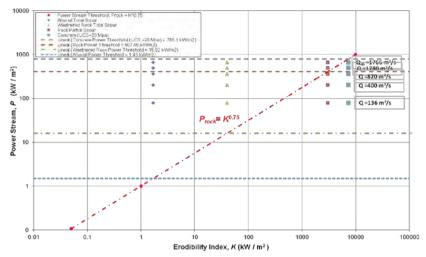
Figure 6. Half-height outlet. Stream power of the jet for different flows as a function of the erodibility: intact rock and concrete cases ( $D_s = 24$  m).
