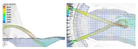
Figure 8. Lateral and top views of the velocity vectors in the pre-excavated stilling basin.
