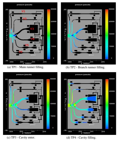
Figure 5- Computed pressure contour along parting surface at different time point (TP) as metal filling the die cavities for modified runner design.
