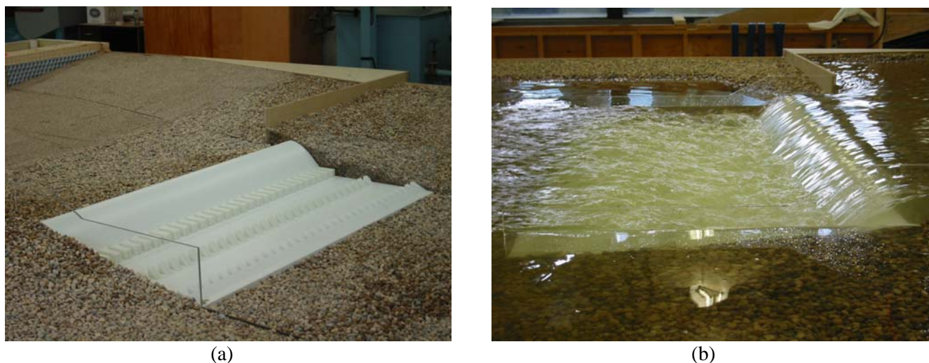
Figure 4: Physical Model (a) Dry (b) Passing design flow
