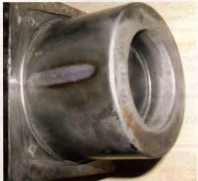
Figure 1a – Moving Core of the Die showing high wear near the gate area.
