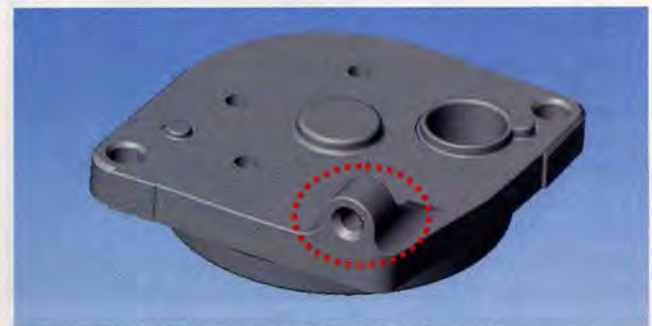
Figure 4a – Model of the part showing the cored hole.
