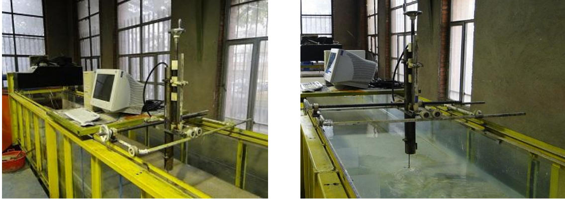
Figure 1. Experimental spur dikes and ADV in Laboratory
