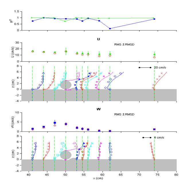
Figure 1. Model-Data comparisons of horizontal and vertical velocities
