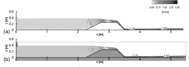
Fig. 11 Velocity contour plots for  $Q = 0.0152 \text{ m}^3/\text{s}$ .
