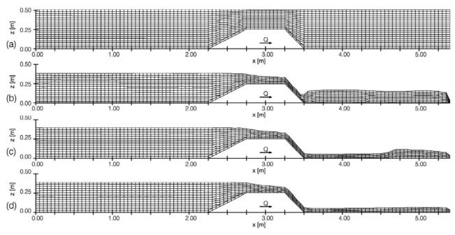
Fig. 5 Free-surface evolution from initial condition (a) to the final free-surface (d) in SSIIM 2. Also the grid after one third (b) and after two third (c) of the computation time is shown. In the computations a finer grid is used.
