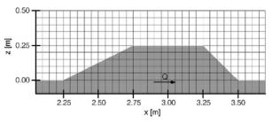
Fig. 2 Sketch of the orthogonal, structured and non-adaptive grid (hexahedral), used in Flow-3D. In the computations a finer grid is used.
