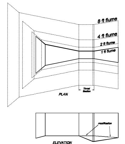
Figure 3. — Details of 1, 2, 4, and 8 ft (0.30, 0.61, 1.22, and 2.44 m) wide Parshall flumes. The elevation view shows the 1-ft flume and the proposed modification of the throat section for converting these structures to long-throated flumes. Note in the plan view the different length-to-width ratios of the throat in each flume.
