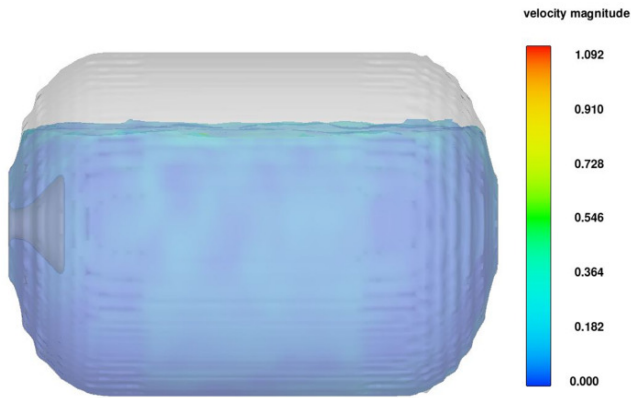
Figure 13: Modelling of propellant sloshing during horizontal transport of the partly filled tank.
