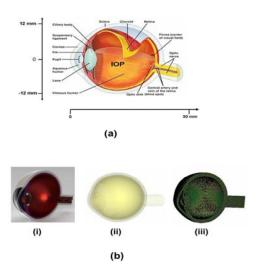
Figure 1. The human eye: (a) interior cross-sectional view showing constituent elements; (b) basic eye geometry, (i) CAD geometry, (ii) 3D STL-based computational geometry, and (iii) sectional view showing computational mesh for structural analysis.
