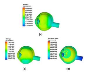
Figure 4. CFD-FSI stress analysis: (a) x-axis stress, (b) y-axis stress, (b) Von Mises stress.
