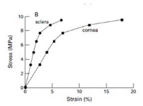
Figure 2. Stress-strain curves ( $\sigma$  vs. $\epsilon$ ) of the sclera and cornea (Uchio *et al.*, 2009).
