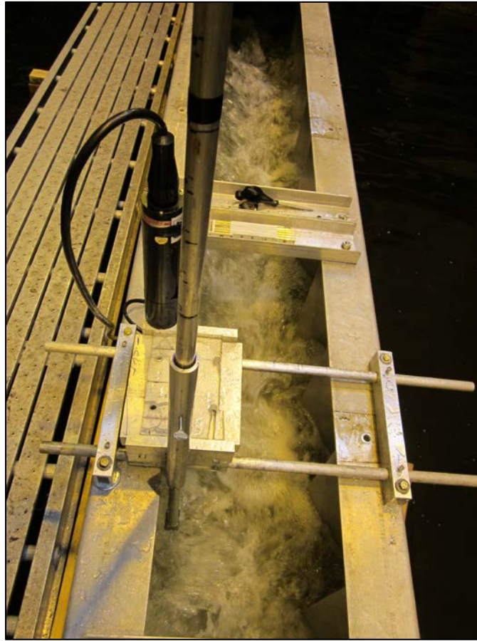
Figure 51: ADV support shown attached to the steppass fishway at the Conte Lab.
