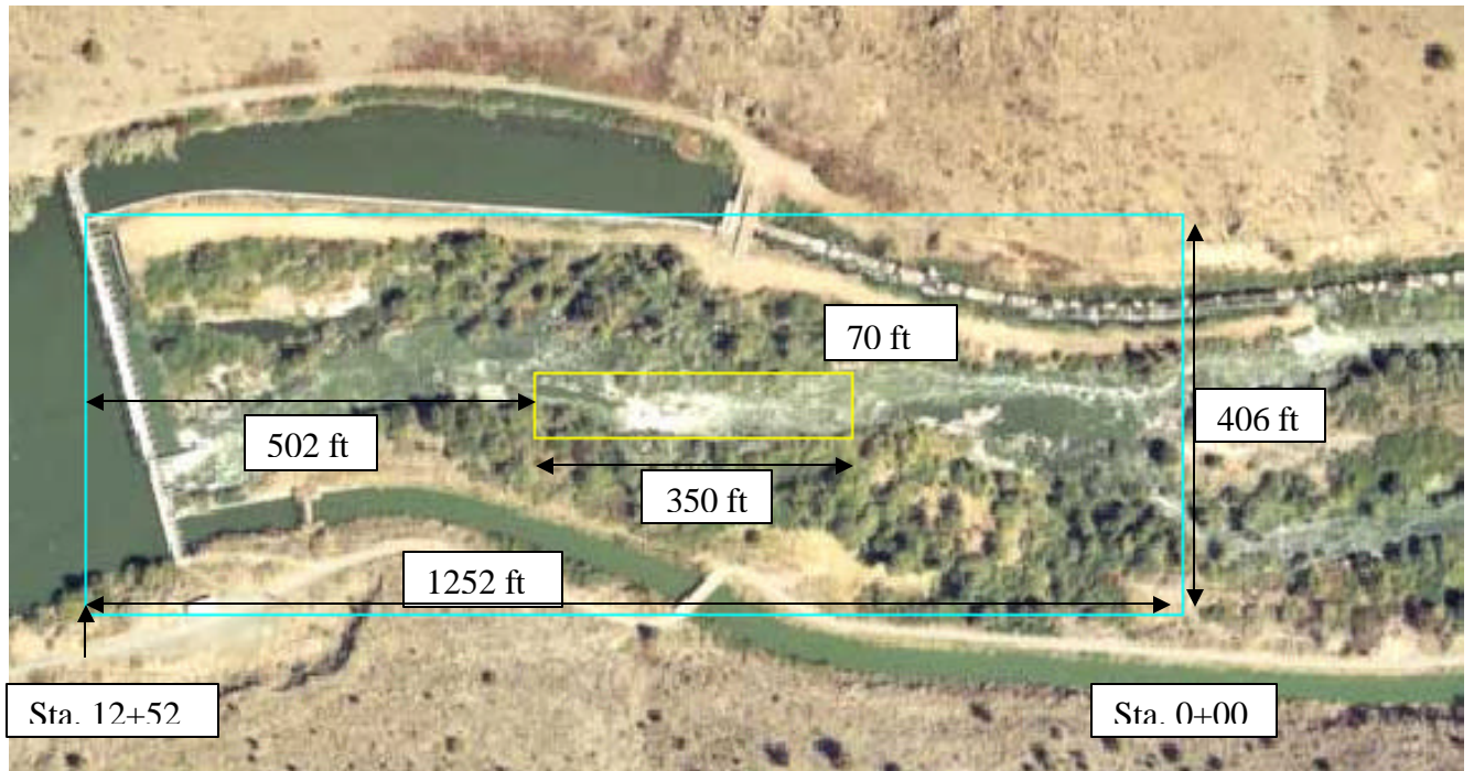
Figure 4 – Numerical model physical boundaries. The area modeled using a single-mesh grid is shown in blue. The falls area modeled using a fine (nested) mesh is shown in yellow.
