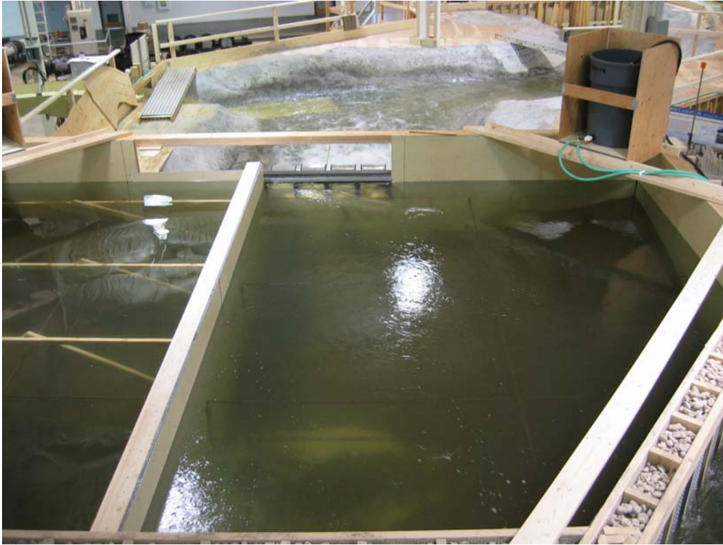
Figure 10. 1:48-scale model with symmetry-boundary wall and 4-gate discharge.
