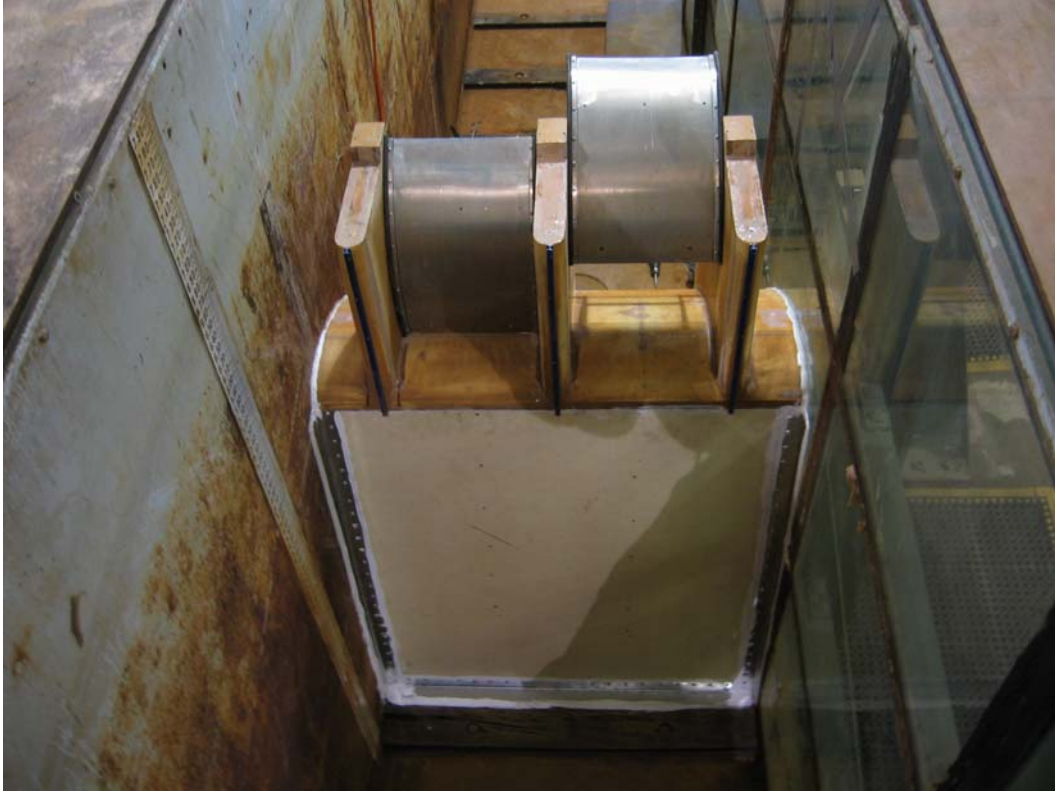
Figure 3. 1:36-scale sectional model under construction in 4-ft-wide flume.
