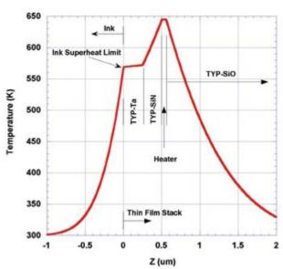
Figure 1: A short electrical pulse is applied to a thin-film stack and superheats the ink.
