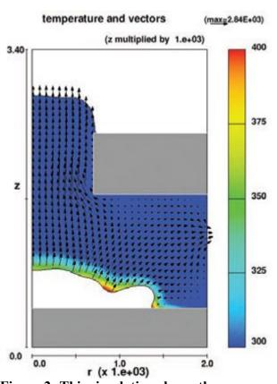
Figure 2: This simulation shows the vapor bubble forming and pushing the ink (blue) through the nozzle plate (top gray block).
