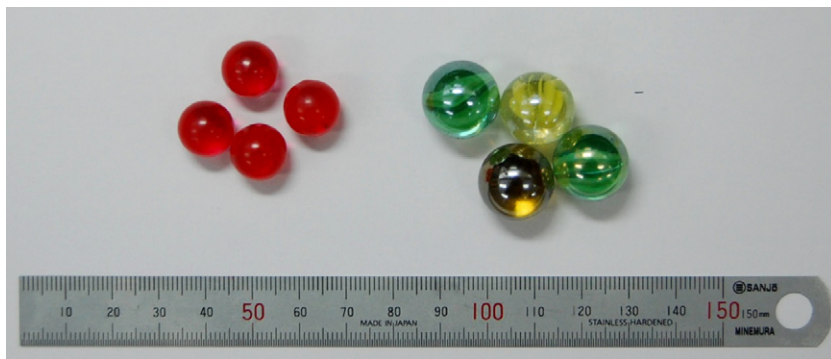
Fig. 8. Debris surrogates (acrylic and glass beads).
