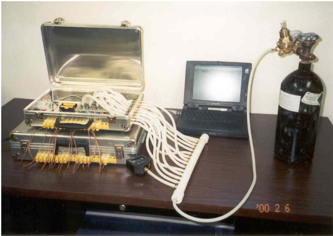
Figure 14. Experimental technique to study pressure losses in core box due to sand deposition in vent area during mold filling process.
