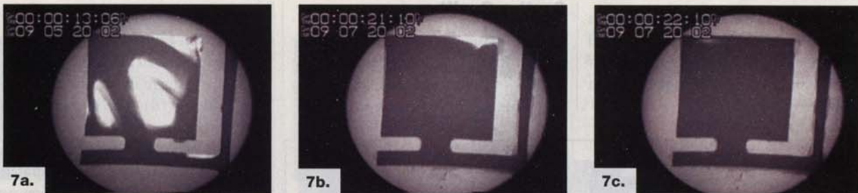
Figure 7: Observations during mold filling; a) cold shot and air entrapment; b) mold gas entrapment during filling; c) Mold gas after metal filing.
