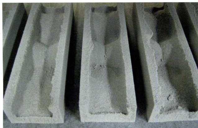
Figure 3: Middle ligament of three generic cores with sand removed in the wet areas
