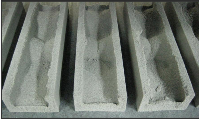
Fig 3. Middle ligament of three generic cores with sand removed in the wet areas.
