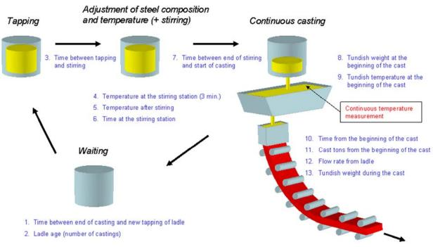
Figure 7 : Neural network inputs from the ladle cycle
