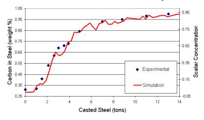
Figure 1 : Measured and calculated carbon content during steel grade change in a tundish
