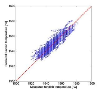
Figure 8 : One example of the simulated and measured results for tundish temperature.
