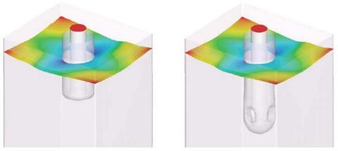
Figure 4 : Electromagnetic stirring dominates the flow in the mould. For instance the shape of the meniscus is almost the same for nozzles No. 3 (straight) and No. 5 (four holes). Casting speed 0.6 m/min.
