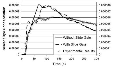
Figure 2 : Comparison of the C-curve results of tundish with no flow modifiers with and without slide gate system
