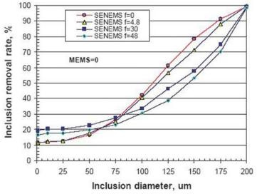
Figure 6 : Effect of SEN-EMS alone on the inclusion removal in the mould; bloom caster; f is the relative intensity.
