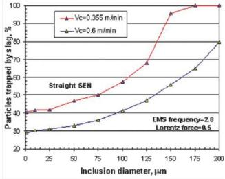
Figure 5 : The casting speed has a clear influence on the separation of the inclusions in the CC bloom mould.
