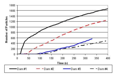
Figure 3 : Number of particles left from the tundish with different flow modifiers
