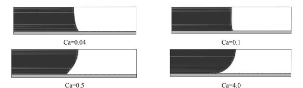
Figure 4. Dynamic contact angle computed as function of capillary number.
