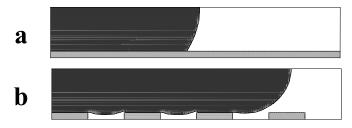
Figure 1. Flow of liquid with static contact angle 120° over (a) smooth surface and (b) a rough surface.
