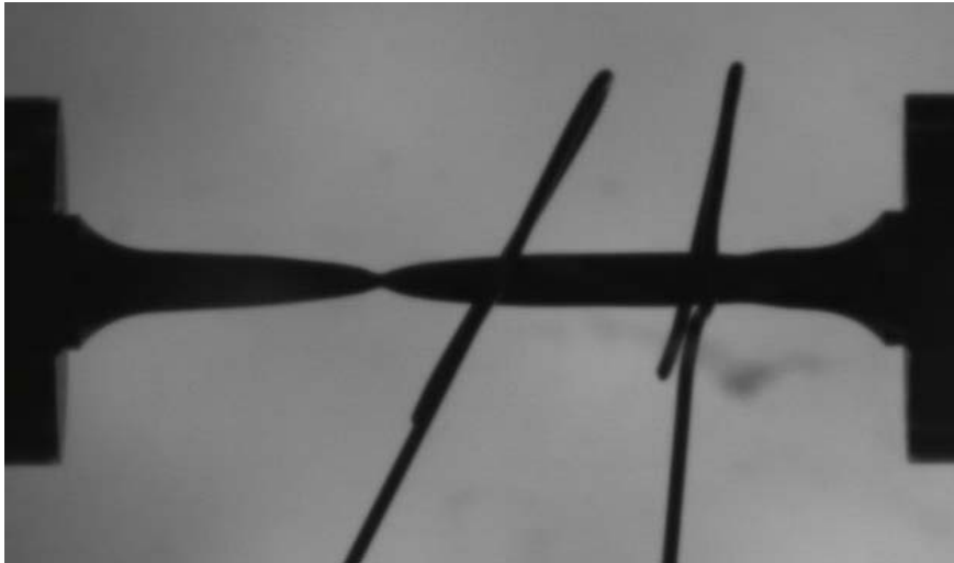
Smooth tensile bar tested in the high beta, 190 ° C, 10 -1 /min
