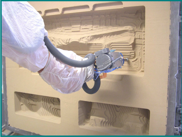
Fig 5. Robotic machining of prototype cars tooling frames in Audi cell at Ingolstadt in Germany
