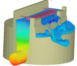
Figure 6 Surface Velocity Contours on CSO
