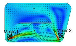
Figure 3 Velocity Contours in Big Canyon Reservoir
