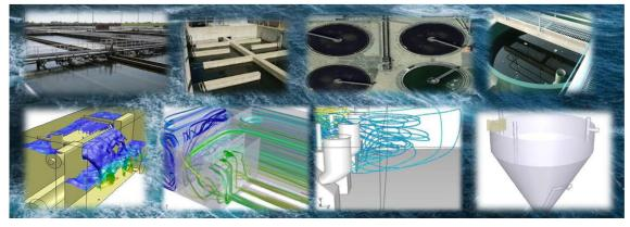
Computational Fluid Dynamics (CFD) is a powerful numerical modelling technique, which is increasingly used to simulate the flow field within process plant and water systems. Typical modelling projects include clarifiers, contact tanks, mixing tanks, pumping station, combined sewer overflow (CSO), reservoirs, pipe loop, thermal plume model and digesters. CFD can provide significant benefits to clients by:
