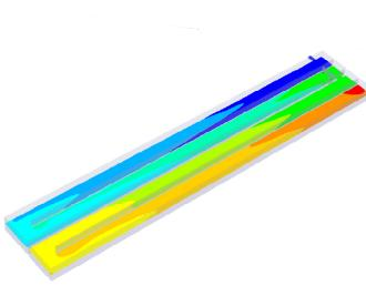
Figure 4 Mean Water Age in Frankley Contact Tank
