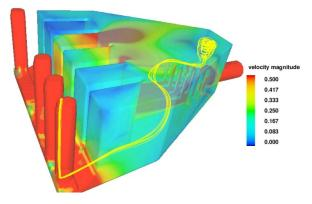
Figure 1 Streamlines inside Pumping Station
