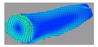
Figure 2 Velocity Contours in a Reservoir
