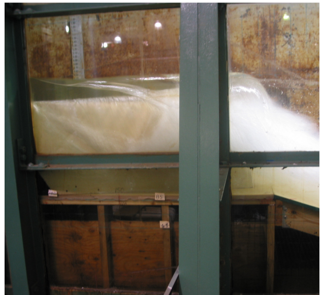
Figure 4. - Flow of 53,000 ft 3 /s over the 25-ft-high labyrinth weir located on the simulated embankment with 3:1 downstream slope leading to the USBR Type II stilling basin.
