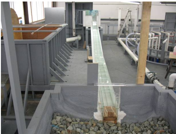
Figure 4: Overall Model Layout from above the tailrace
