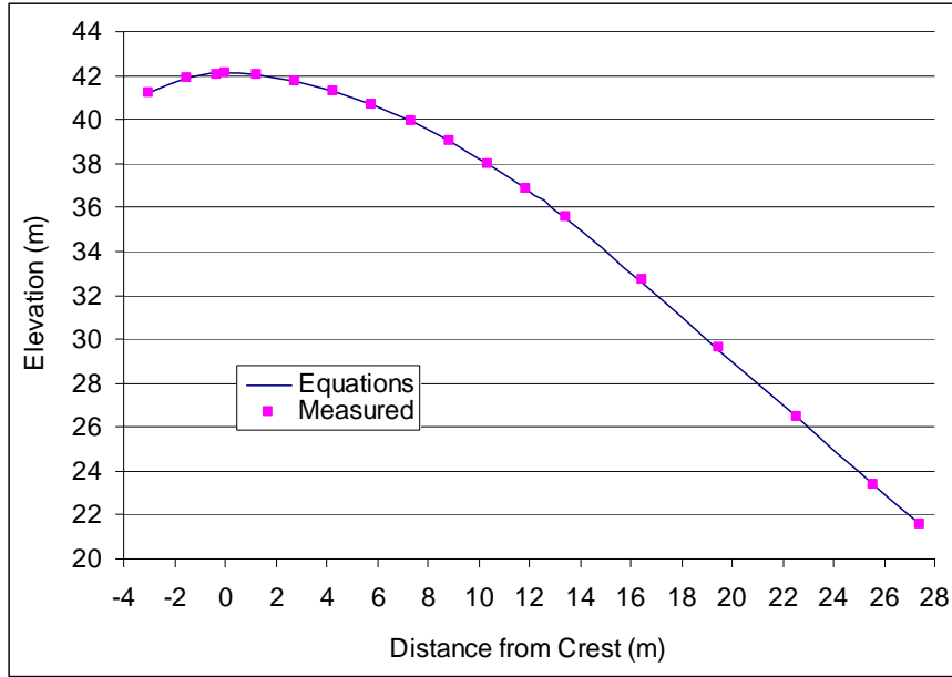
Figure 4.4 Verification of water surface profile measuring device by comparing the measured spillway surface with design equations.
