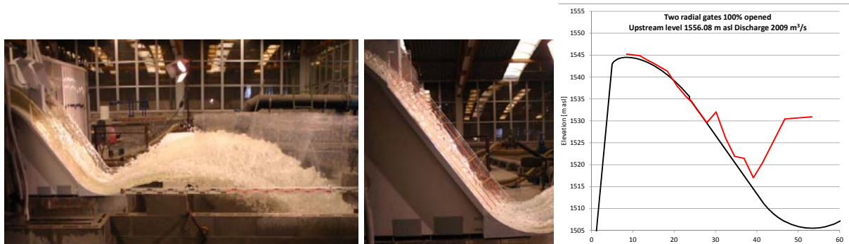
Fig. 7. Jet trajectories (left), water elevation along the surface spillway (centre), pressure acting over the chute (right).
