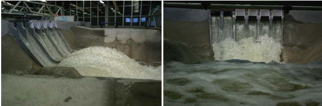
Fig. 5. Hydraulic preliminary tests. reproduction of the PMF (approx. 12'000 m 3 /s)
