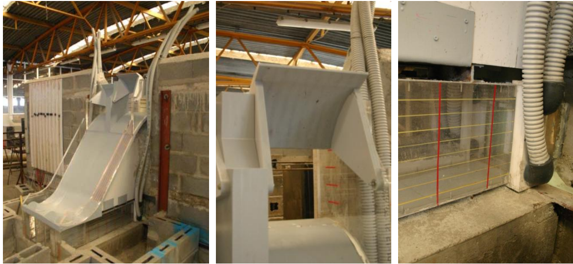
Fig. 3. 1:40 scale model of the surface spillways (left) equipped with radial gates (centre) and bottom outlet.
