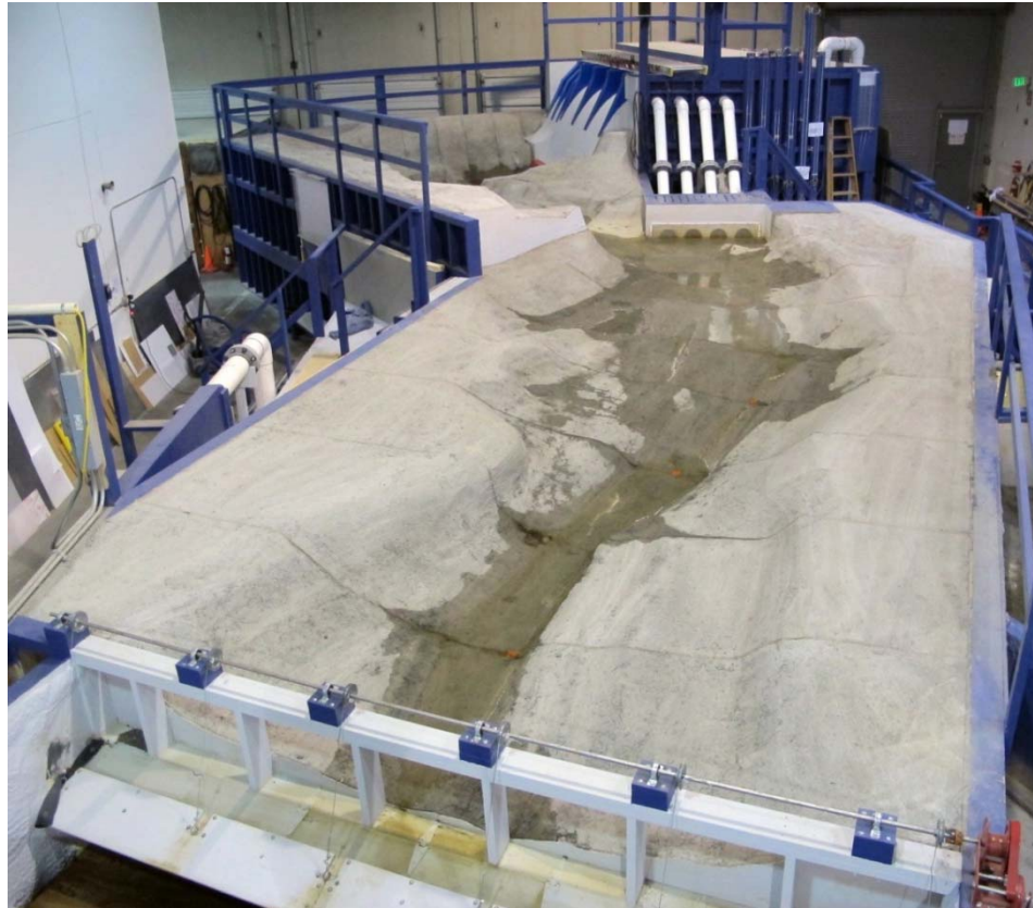
Figure 10 – 1:30 Scale Physical Model of Long Lake HED
