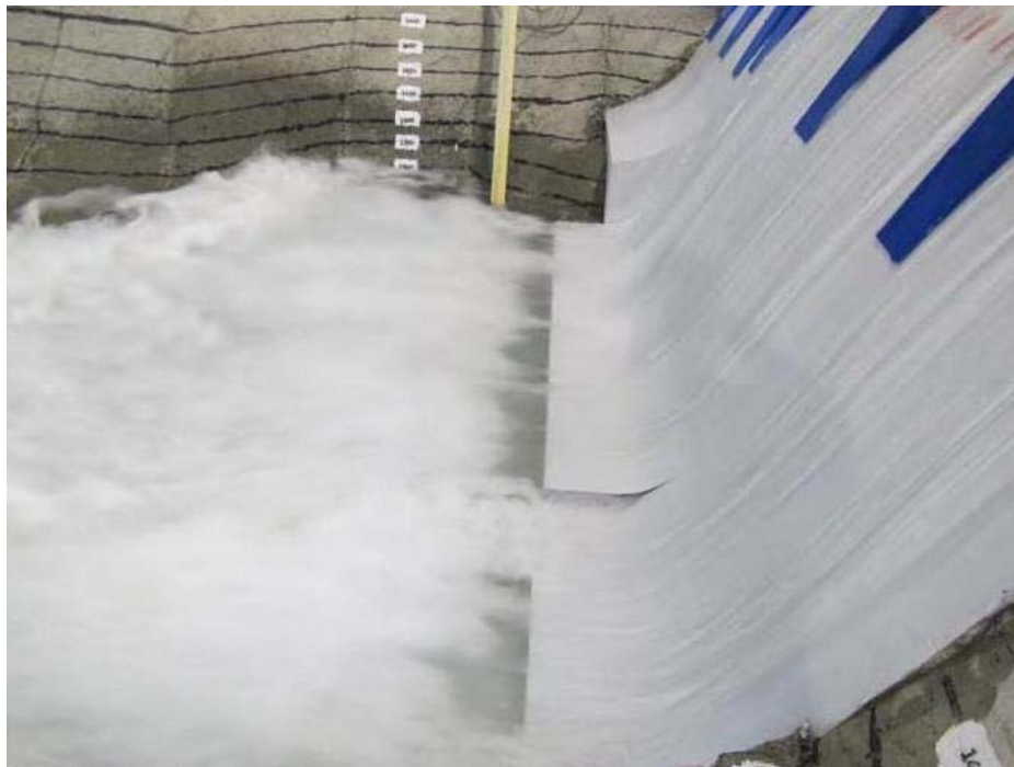
Figure 15 – Alternative 1 (Final Configuration) Skimming Flow at 11,900 cfs total river flow (5,000 cfs through spill bays 7 and 8 only + powerhouse flow of 6,900 cfs)
