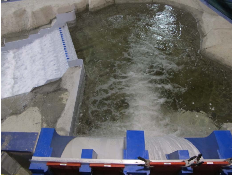
Figure 12 – Alternative 6 Stepped Spillway (upper left of photo)
