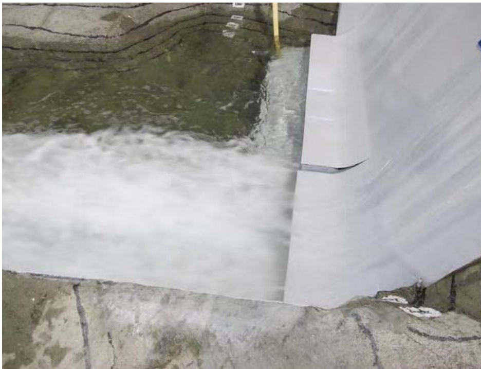
Figure 15 – Alternative 1 (Final Configuration) Skimming Flow at 11,900 cfs total river flow (5,000 cfs through spill bays 7 and 8 only + powerhouse flow of 6,900 cfs)
