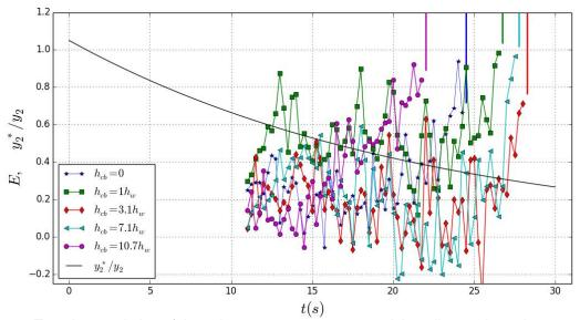
Figure 4. Transient evolution of the submergence parameter and the tail water boundary condition. Solid vertical wider lines mark off the sweep off time value.
