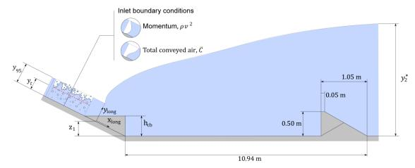
Figure 1. Stilling basin geometry and inlet boundary condtions.
