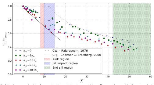
Figure 3. Maximum velocity decay starting at the toe position. Comparison with the classic turbulent wall jet (Rajaratnam, 1976) and the Classic Hydraulic Jump data (Chanson, 2000).
