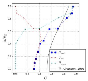
Figure 2. Air concentration profiles at the stilling basin inlet section.
