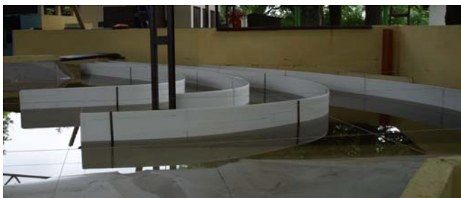
Fig. 5. PVC guiding walls: Correction applied to the physical model in order to reach hydraulic similarity of the velocity field between model and prototype.
