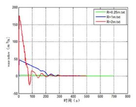
Figure 13: Change curve radius of water inflow rate and the time of water inrush
