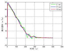
Figure 16: Water inflow rate curve of groundwater characteristics change with time
