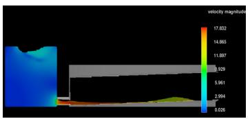
Figure 11: The total water inflow velocity profile
