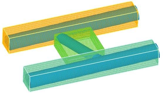
Figure 1: FAVOR calculation model of FLOW-3D
