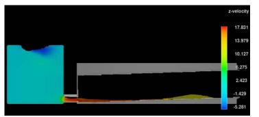
Figure 10: Velocity profile along the axis of tunnel
