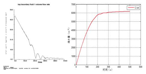
Figure 3: Water inrush water inflow rate with time Figure 4: Water gushing quantity change with time
