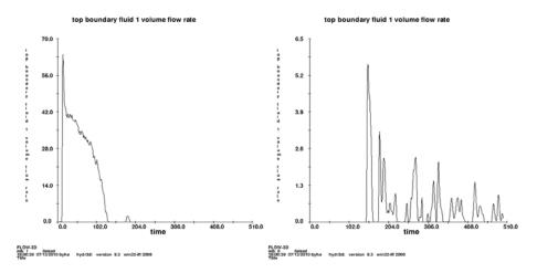
Figure 7: Left line tunnel drainage rate changes with time Figure 8: Right line tunnel drainage rate changes with time
