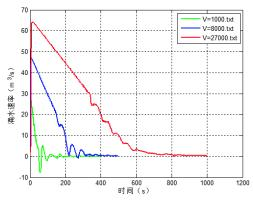
Figure 15 Variable flow rate and time curve of sudden water scale
