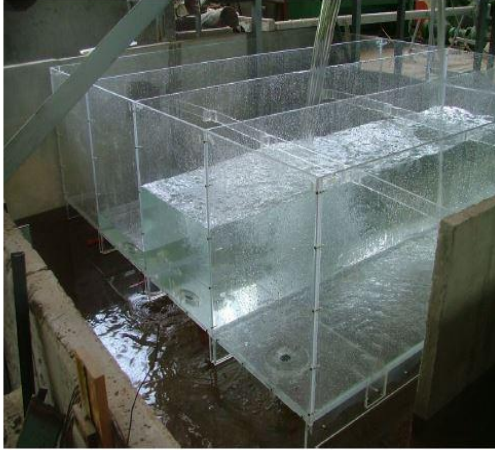
Figure 5.8a Experimental Setup (Channels under Grates)
