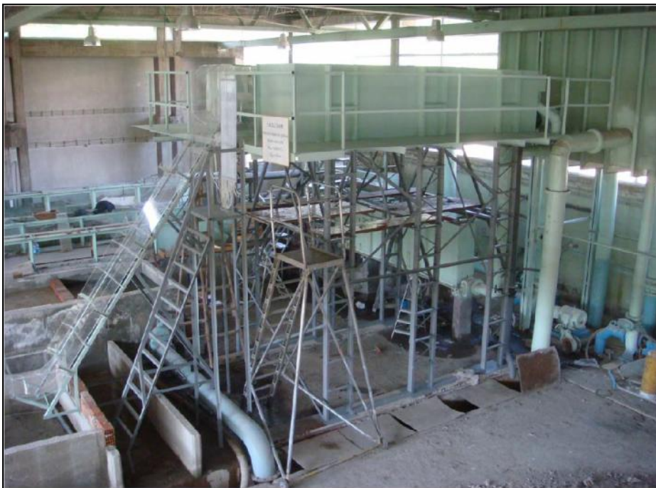
Figure 2.2 Hydraulic Model of Laleli Dam Spillway
