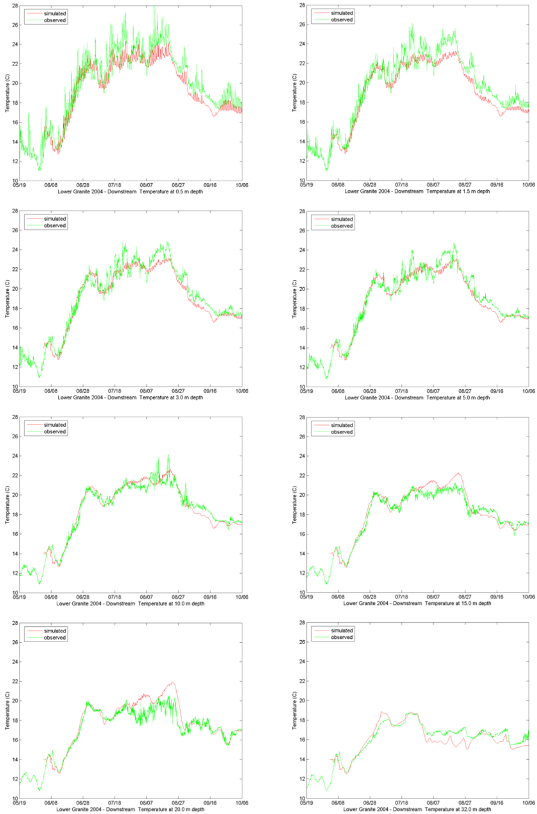
Figure C.14 Observed and Simulated temperatures at LWG forebay BRZ, 2004
