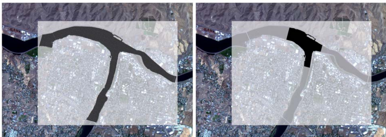
Figure 4.16. Extent of the coarse (left) and fine (right) domain 3D confluence zone model
