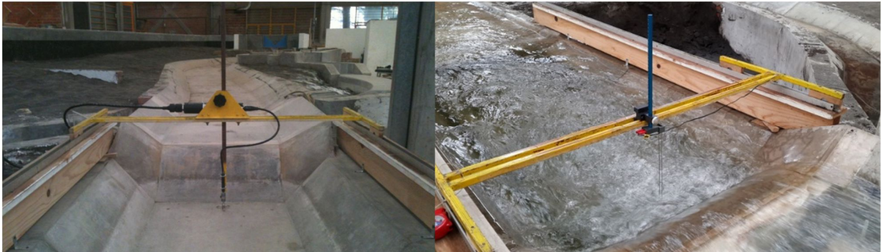
Figure 2 Instrumentation with Micro ADV and limnimeters
