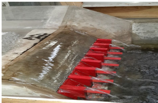
Figure 7. Trial Spillway with deflectors
