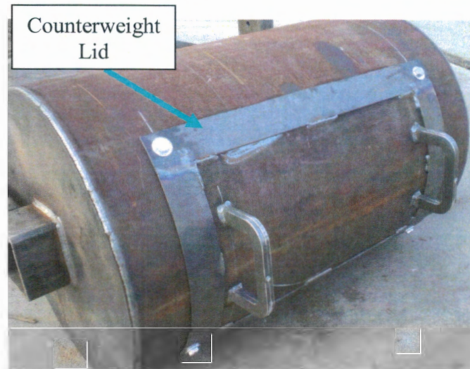
Figure 19. ITRC Flap Gate counterweight lid
