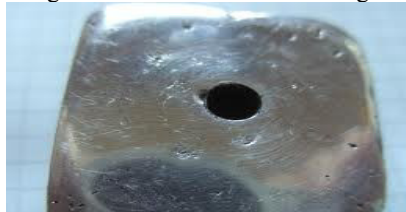
Figure 2: Blow holes on casting
