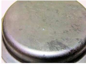
Figure 1: Flow mark on casting
