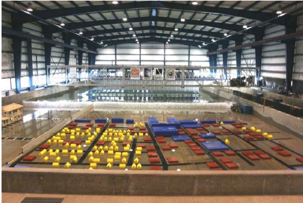
Figure 4.93 Photograph of 1:50 scale model of the town of Seaside, Oregon constructed in the Tsunami Wave Basin at OSU (Cox et al., 2008; Rueben et al., 2011).
